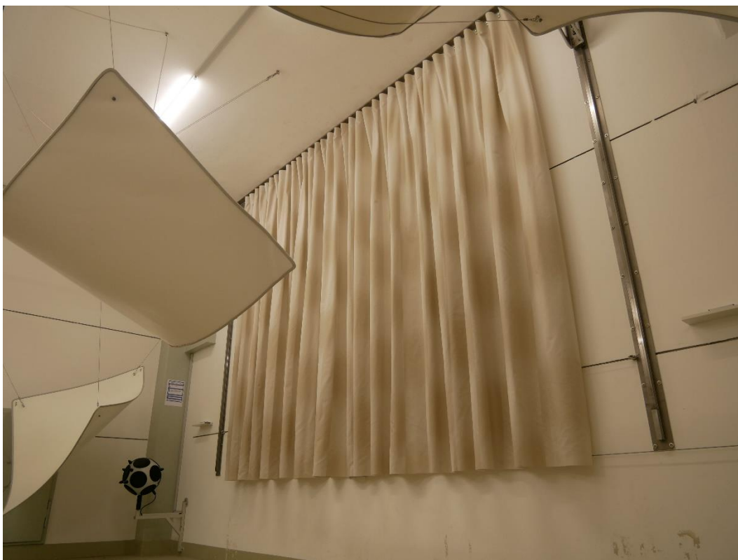
Figure B.4. Pleated hanging curtain, 100 % fullness in the reverberation room: diagonal view.
